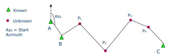
Figure A-2, type II, Close traverse to single Known point at the end
