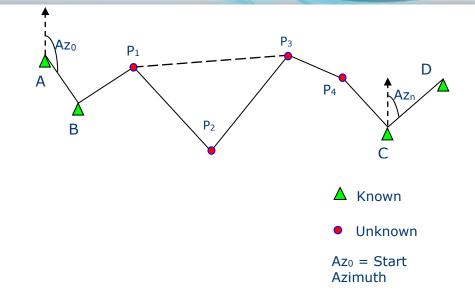
The least square traverse adjustment process automatically identify all the possible connections and equations. The meaning of minimum least square solution is that the sum of the adjustments squares must be the minimum possible.
