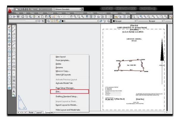
24. In the 'Plot' window, define the printer's name and make sure that the paper size is changed from 'ISO A4 (210.00 x 297.00 MM)' to 'A4'.
