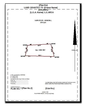
21. In order to move the plan in the layout, double click on the layout within the plane's area. A border will be displayed. Use AutoCAD 'Pan' button S
