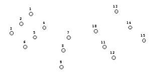
In this drawing area the contour lines will be calculated also in the confined area between the following points 1<-13<-10<-7<-4<-1, and not as we might have preferred, without this area. To calculate the contour lines without this area, you must define it in the following manner :
