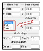
Note : the grid, made by 3 points (Pick option) or Polyline (Select option), must include the whole area for calculation (including the border made by Polyline or Pick option).
