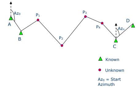
Figure A-3, type III, Close polygon to 2 Known points at the end
